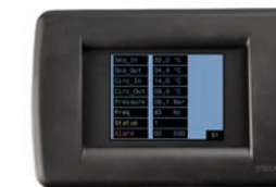
Chiller status display
